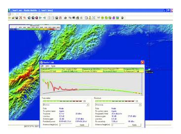
Figure OI 3: Profile of a 280 km path over which standard WiFi gear with OpenWRT firmware which allows for the ACKtimeout increase was used to transfer files at about 65 kb/s in April 2006 between Pico del Aguila and El Baul in Venezuela.
