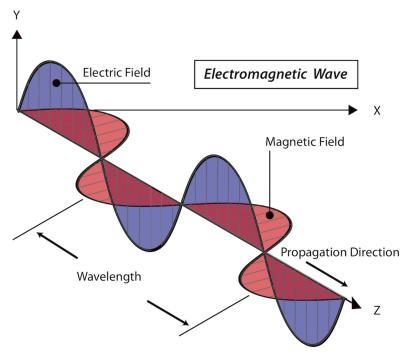
Figure RP 3: Vertically polarized electromagnetic wave
