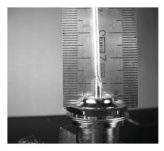
Figure AC 27: The length of the wire is critical. Unscrew the nut from the connector, leaving the washer in place. Insert the connector into the hole of the can. Screw the nut on the connector from inside the can.
