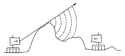
Figure RP 9: Diffraction over a mountain top.
