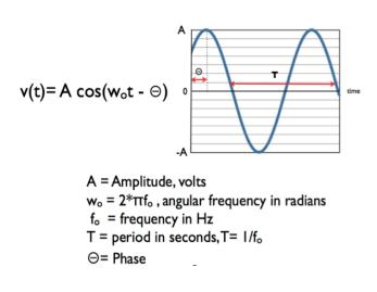
Figure TB 6: Sinusoidal Carrier Signal
