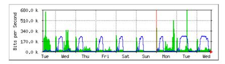
Figure NM 22: The classic network flow graph. The green area represents inbound traffic, while the blue line represents outbound traffic. The repeating arcs of outbound traffic show when the nightly backups have run. Traffic patterns will vary with what you are monitoring.
