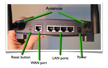
Figure HW 5: Linksys Access Point
