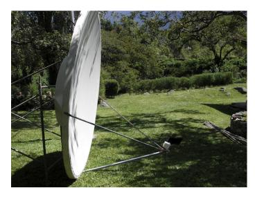
Figure CsLD 4: 2.4 m offset fed reflector with a 12 dBi antenna at its focus, looking 14° down. The actual elevation is 8° up.
