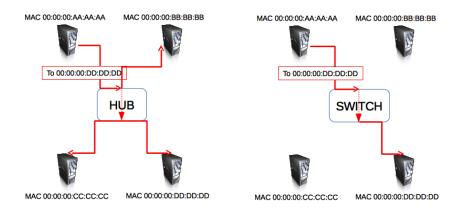
Figure NG 14: A hub simply repeats all traffic on every port, while a switch makes a temporary, dedicated connection between the ports that need to communicate.
