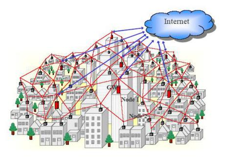
Figure MN 1: A metropolitan area mesh network, providing local connectivity and Internet access via multiple Internet gateways
