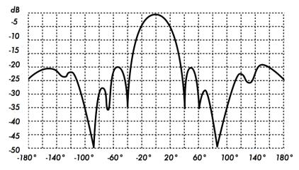
Figure ATL 7: A rectangular plot of the radiation pattern of a Yagi antenna.
