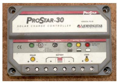
Figure OGP 3: A 30 Amp solar charge controller
