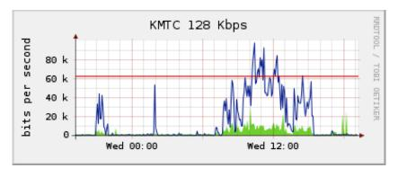
Figure NM 2: Polling the edge router can show you the overall network utilisation, but you cannot break the data down further into machines, services, and users.
