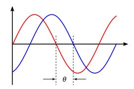
Figure RP 2: Phase Difference between Two Waves
