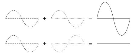
Figure RP 10: Constructive and destructive interference.
