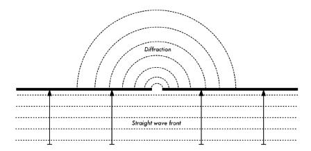
Figure RP 7: Diffraction through a narrow slit.
