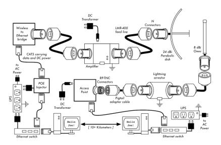
Figure HW 1: Common Interconnects and Components for a Wireless PtP link.
