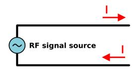
Figure ATL 2: Bifilar transmission line
