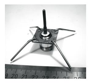
Figure ATL 11: Quarter wavelength ground plane antenna.
