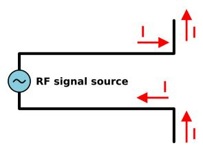
Figure ATL 3: Antenna from transmission line
