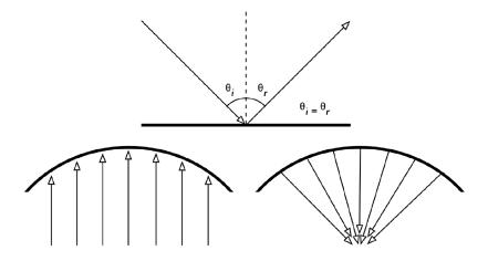
Figure RP 6: Reflection of radio waves. The angle of incidence is always equal to the angle of reflection. A metal parabolic surface uses this effect to concentrate radio waves spread out over it in a common direction.
