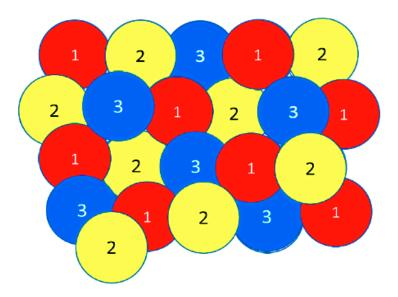
Figure RS 1: Cellular sharing of spectrum
