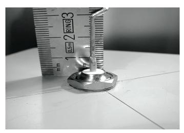
Figure AC 14: The first coil should start 3.0 cm from the surface of the plate.
