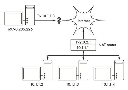
Figure NG 13: Network Address Translation allows you to share a single IPv4 address with many internal hosts, but can make it difficult for some services to work properly.
