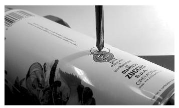
Figure AC 23: Mark the hole before drilling.
