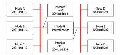
Figure NG 8: Two separate IPv6 networks.
