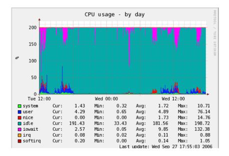
Figure NM 25: RRDtool can show arbitrary data, such as memory and CPU usage, expressed as an average over time.
