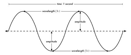
Figure RP 1: Wavelength, amplitude, and frequency. For this wave, the frequency is 2 cycles per second, or 2 Hz, while the speed is 1 m/s.
