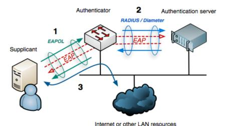
Figure SWN 4: The use of 802.1X with tunnelled EAP for network access (courtesy SURFnet)
