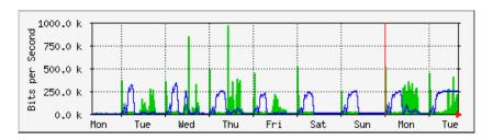
Figure NM 18: The same network logged over an entire week reveals a problem with backups, which caused unexpected congestion for network users.
