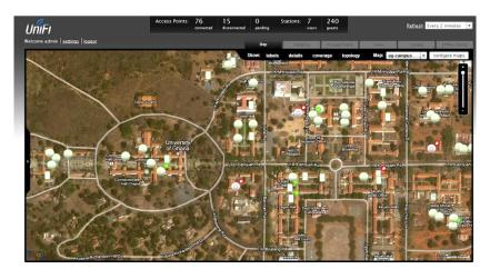
Figure CSG 6: Layout of University of Ghana campus with AP's.
