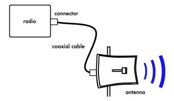
Figure ATL 1: Radio, transmission line and antenna
