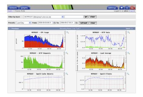
Figure NM 10: Cacti can manage the polling of your network devices, and can build very complex and informative visualisations of network behaviour.
