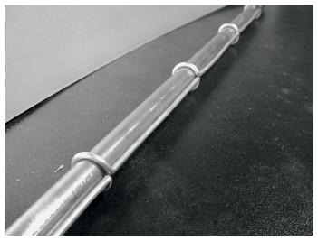
Figure AC 8: Inserting a pipe can help to straighten the wire.
