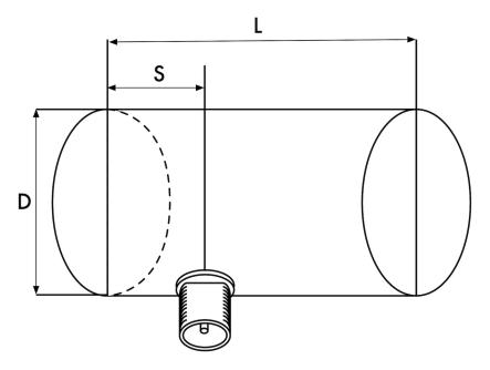
Figure AC 19: Dimensional constraints on the cantenna
