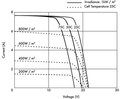
Figure OGP 7: Different IV Curves. The current (A) changes with the irradiance, and the voltage (V) changes with the temperature.
