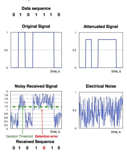
Figure TB 5: detection of a noisy signal
