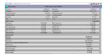
Figure OI 5: Results of the Radio Mobile on-line simulation for the 380 km link between Aguila and Platillon.
