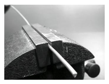
Figure AC 2: Make the wire as straight as you can.
