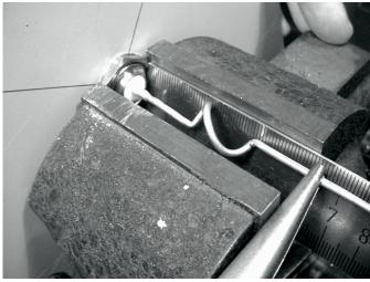
Figure AC 15: Stretching the coils. Be very gentle and try not to scrape the surface of the wire with the pliers.
