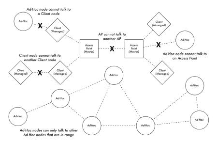
Figure WF 1: APs, Clients, and Ad-Hoc nodes.
